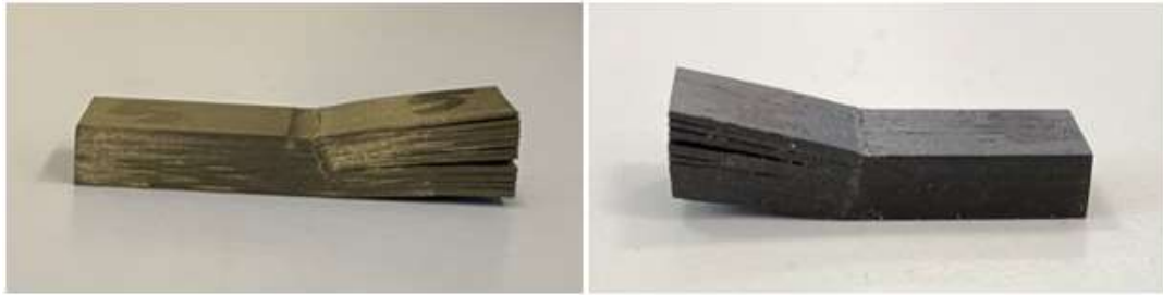
Figure 3.4 Examples of the interlaminar shear failure mode of the specimens.
