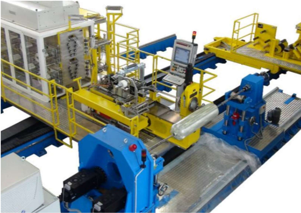
Figure 2.2 General view of the filament winding system.
